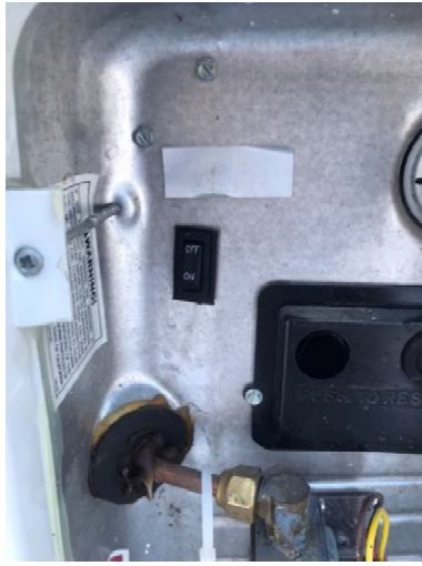
Hot water tanks switch on the outside
